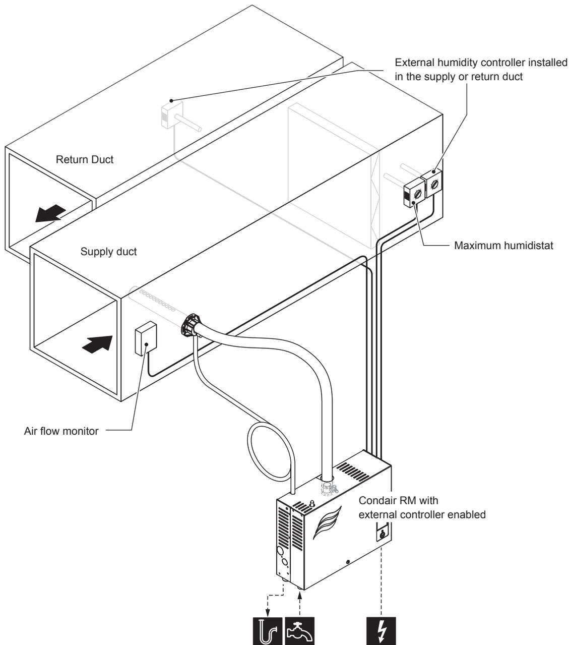
Fig. 5: System layout for operating the Condair RM with a demand signal from an external humidity controller
