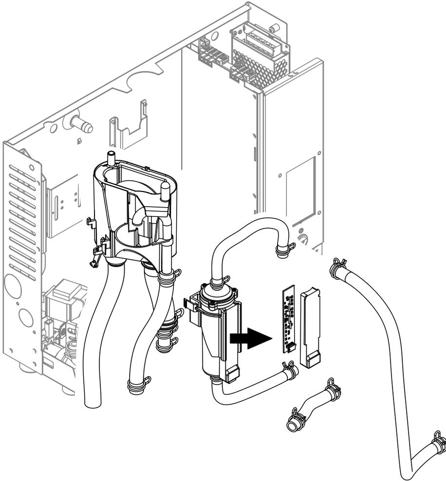
*Fig. 8: Removal of the filling cup, the level unit and the water hoses*
