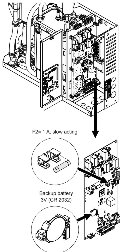
Fig. 17: Position of the backup battery and the fuses on the control board
