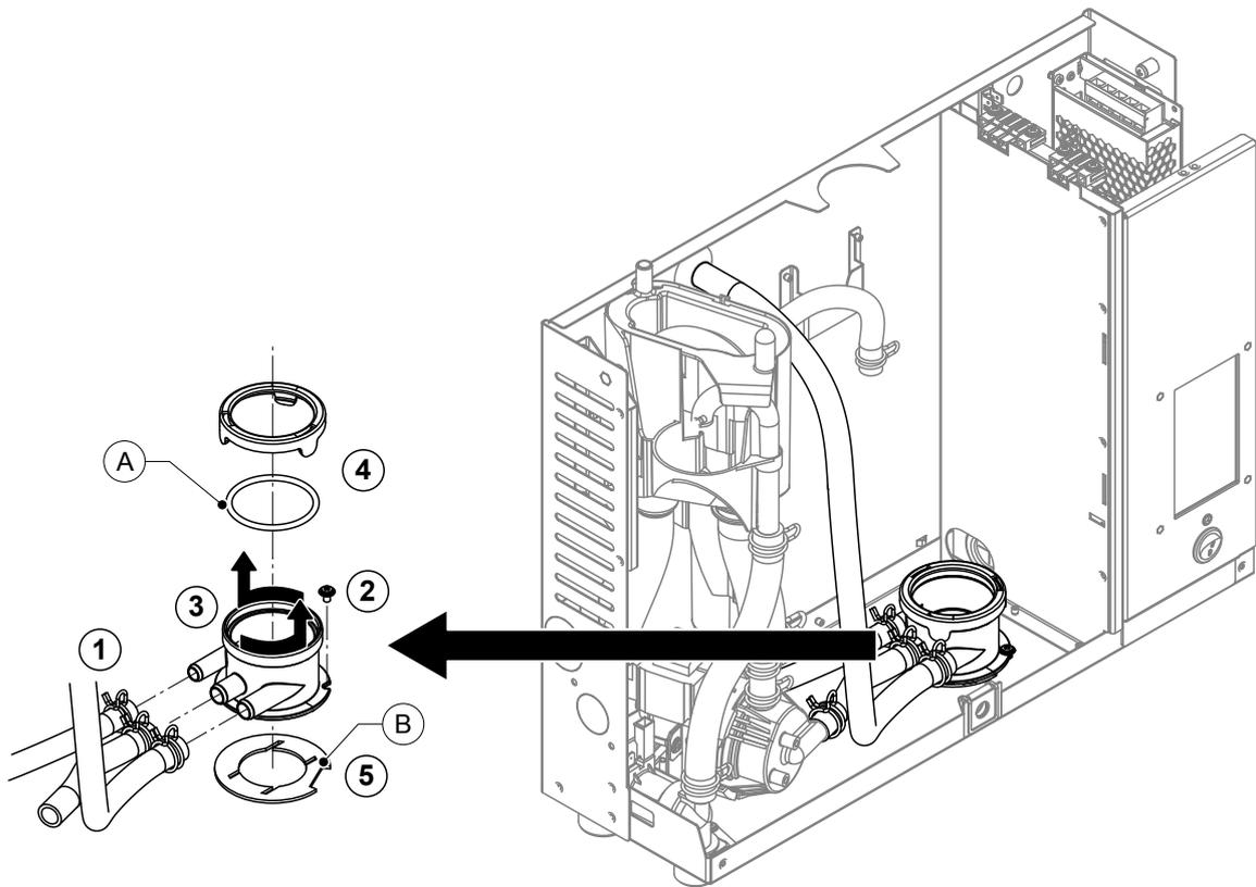
*Fig. 12: Removal of the steam tank receptacle*
