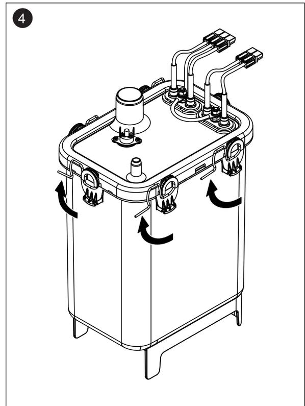
3. Carefully lift the steam tank out of steam tank receptacle and remove it towards the front of the steam humidifier.
