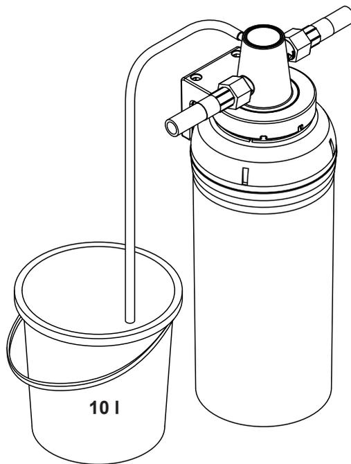
Fig. 14: Lead bypass hose into an empty container
